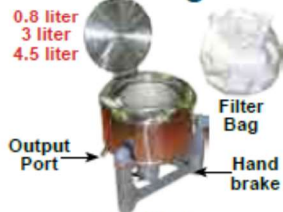
BSCEN-600 • Speed range: up to 3000rpm • Max. RCF: 1509G • Capacity: 800ml, 3L, 4.5L. • Basket size: diam. 150mm H80mm.
