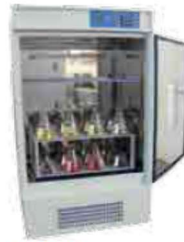
LOM-560D Dual Shaking Platform 480x600mm
